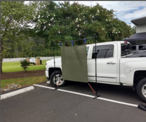
Nine Panel Velcro imaging blanket for large mosaic scans. Includes adjustable mounting frame (as seen in picture) which allows scanning in tightest places with lowest dead area from sides and bottom
